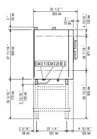
CWII Cold Water inlet 1 (cleaning) = Cold Water Inlet 2 (steam generator) CWI2
